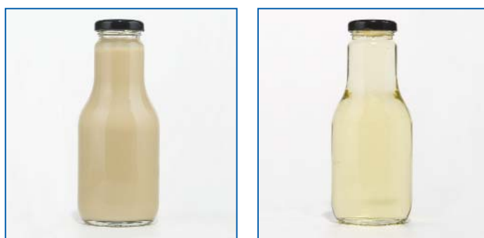
Figure 4: Lees before filtration (left), and recovered wine after filtration (right).
